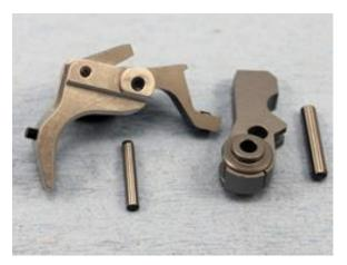
Anyhow, I have a couple of these housings so I decided to try it out on one instead of the common black polymer trigger housing. The KIDD drop-in trigger job kit installed without any issues. Using my Wheeler Engineering trigger pull gauge it measured 1.75-pounds.
